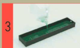
Pour the diluted solution into the trough. Do not overfill!
