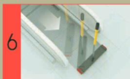
Place the device onto the moving treads, allow it to align with the combs and drop into place.
